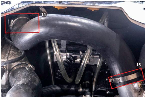
5. Cut and remove the zip ties shown before moving the hoses out of the way.
