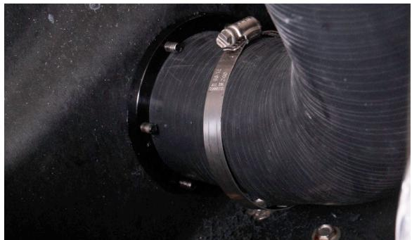
**16.** Attach the hose from the waterbox to the new outlet and use OEM hose clamps to fasten each end securely.
