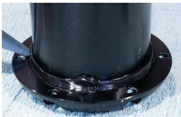
**15.** Place the retainer ring behind the outlet hole and slide the exhaust outlet through it. Begin lightly tightening the bolts through the outlet and ring a little at a time before finally securing them tightly.
