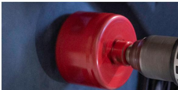
**13.** Place the Worx Exhaust outlet through the whole and ensure it is rotated as pictured below. Holding the outlet firmly, use a 6mm to drill out your bolt locations.
