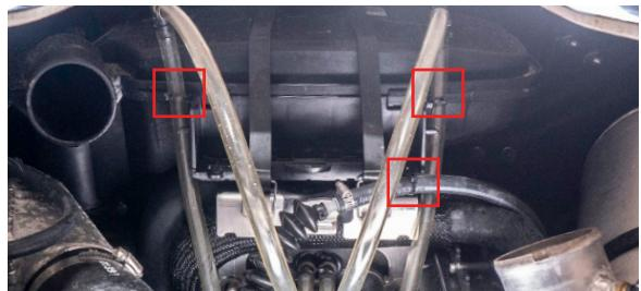
6. Unclip the straps securing the resonator box in place.
