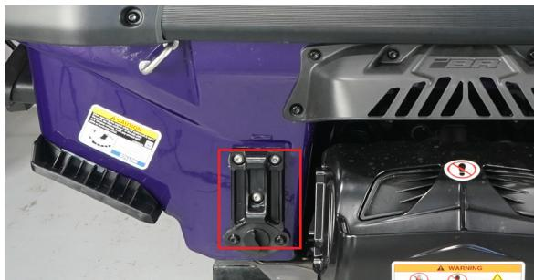
**10.** Line up the template (page 4) with the three holes from the ladder attachment.
