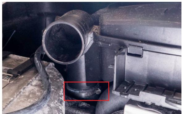
**8.** Place the exhaust block off cap in the OEM exhaust outlet hose before retightening the hose clamp.
