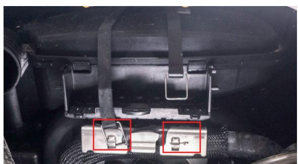
7. Undo hose clamp<sup>(16)</sup> pictured before removing the resonator box.
